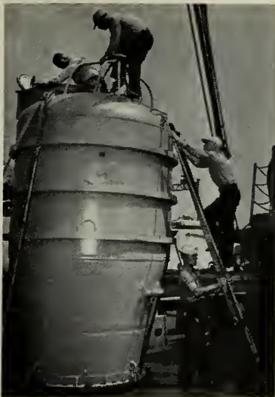
THIS WAY OUT—Sub rescue bell is shown on deck of USS Tringa (ASR 16) and (right) as a cutaway scale model.
